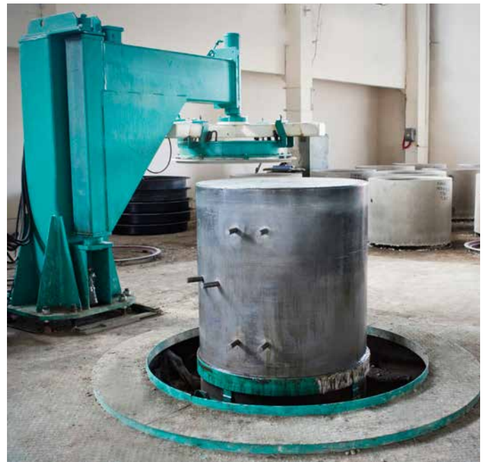
Mould equipment Inner mould and outer mould with accessories and the lifting beam useful for the handling. Vibrating system with central vibrators mounted in the mould core, optional with frequency converter.
